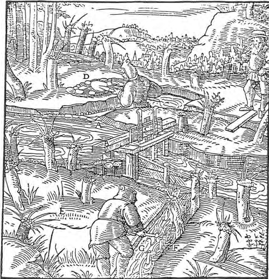
A—RIVER. B—WEIR. C—GATE. D—AREA. E—MEADOW. F—FENCE G—DITCH.
