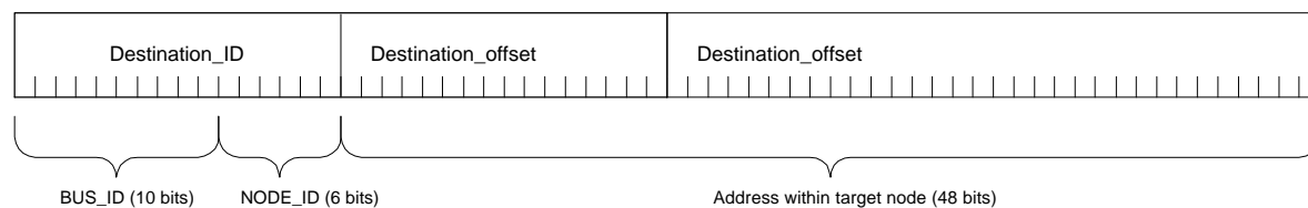
Figure 13: Destination addressing within asynchronous packet format
