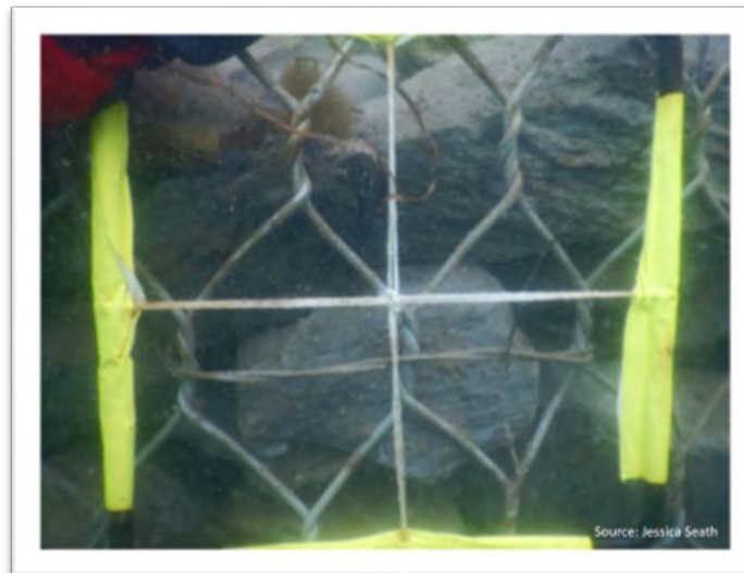
Figure 3.1: The 0.2 x 0.2 m stainless-steel metal quadrat lined with yellow tape used for conducting invertebrate and algae surveys, shown on the vertical surface of a gabion habitat in Knysna Harbour.
