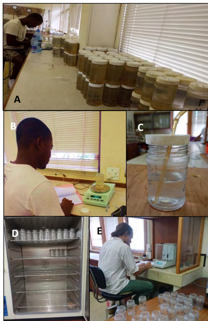
Figure 5-5 A: Settling samples, B: weighing whole sample, C: removing supernatant, D: oven drying and E: weighing empty jars during the laboratory SSC analysis
