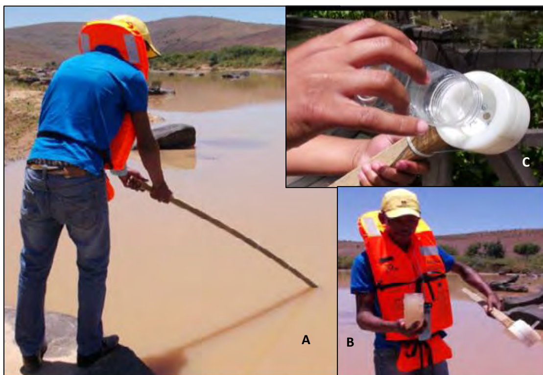
Figure 5-2: citizen technician sampling (A and B) at the riverbank with an isokinetic pole-and-jar sampler. C shows the 450 ml plastic jar being screwed into the head assembly of the wooden pole (Bannatyne et al., 2017).
