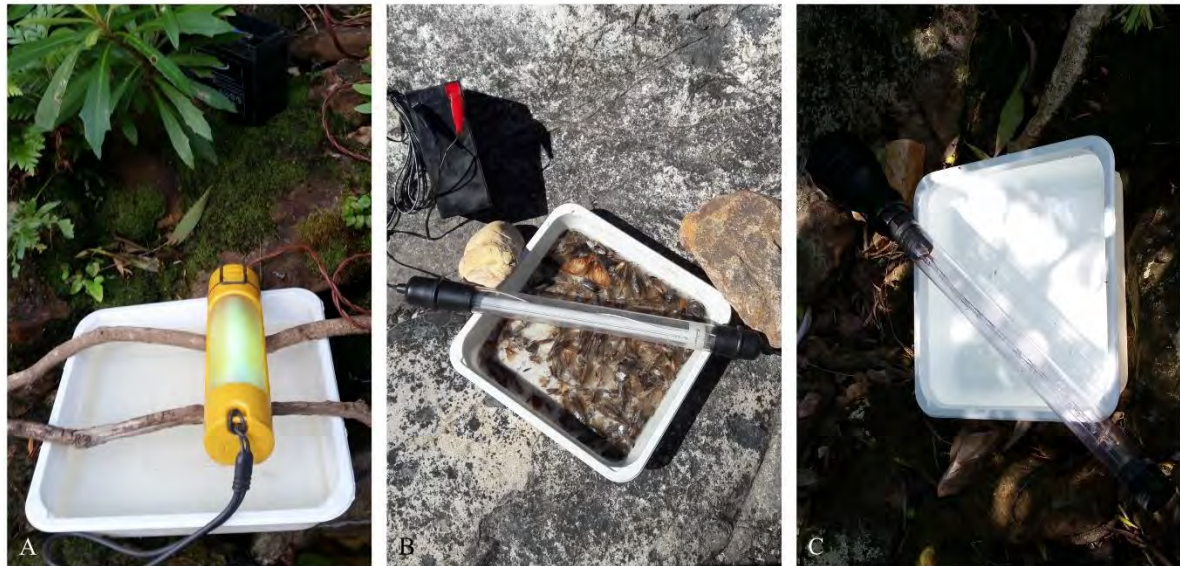
Figure 3.1 The different UV light sources that was used with the pan light trap method for collecting adult mayflies: A) 6 V, B) 12 V, C) LED. © IS Ferreira.
