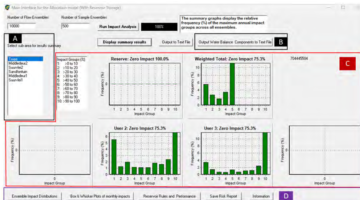
Figure 3.10: Risk tolerance interface of the Water-Sharing Tool for each user and the community within a sub-basin (A, C). Hydrological impacts of reservoir storage and surface water withdrawal are given by the water balance component output (B). Uncertainty assessment of impacts is explored using the summary outputs in D.
