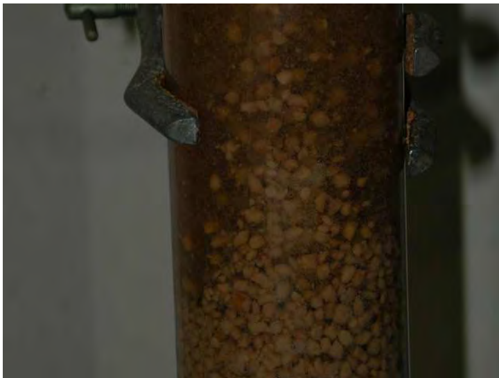
Figure 5. 16 The transitional zone at the top of the packed bed, where support particles are fluidised by rising carbon dioxide bubbles. (Photograph J. Cambray)
