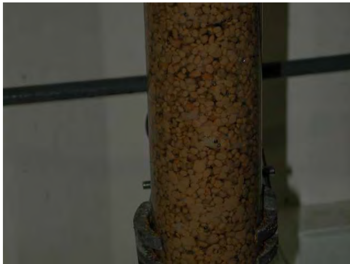
Figure 5. 15 The packed bed region of the glass tower bioreactor. Note how the yeast has formed semi-spherical biofilm particles around the 2 mm cubed root particles. The gas which evolved as a function of fermentation is visible in the spaces between supports. (Photograph J. Cambray)
