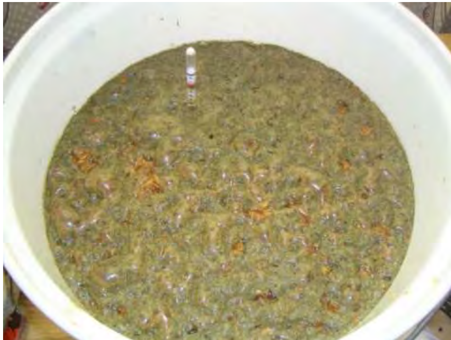
Figure 2. 18 The bioreactor after 2 hours of fermentation. Vigorous carbon dioxide gas evolution was evident. Note the hydrometer which was used to provide a rough indication of the rate of fermentation to allow appropriate biomass sample taking.
