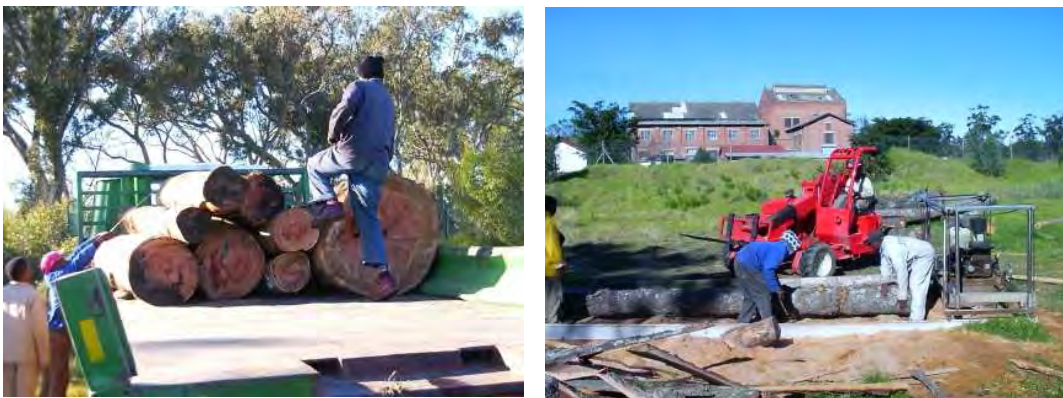
Figure 7.9 The sawmill converted low quality logs as seen on the left into timber using a portable Petersen sawmill unit seen in operation on the right. The process was labour intensive.
