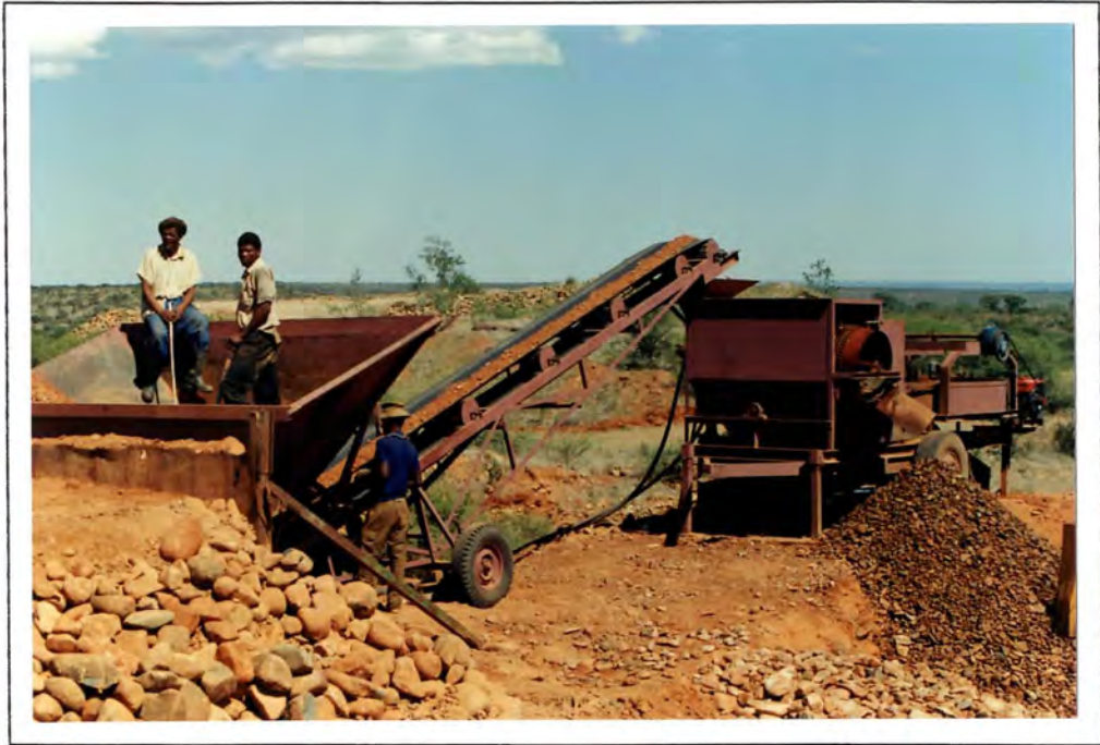
PHOTO 3 : Typical, small-scale digger's rig with washing pan at Longlands.
