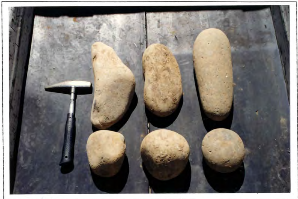
PHOTO 23 : Visual determination of roundness. From left to right: rounded (49-60), well rounded (60-75) and very well rounded (75-85).
