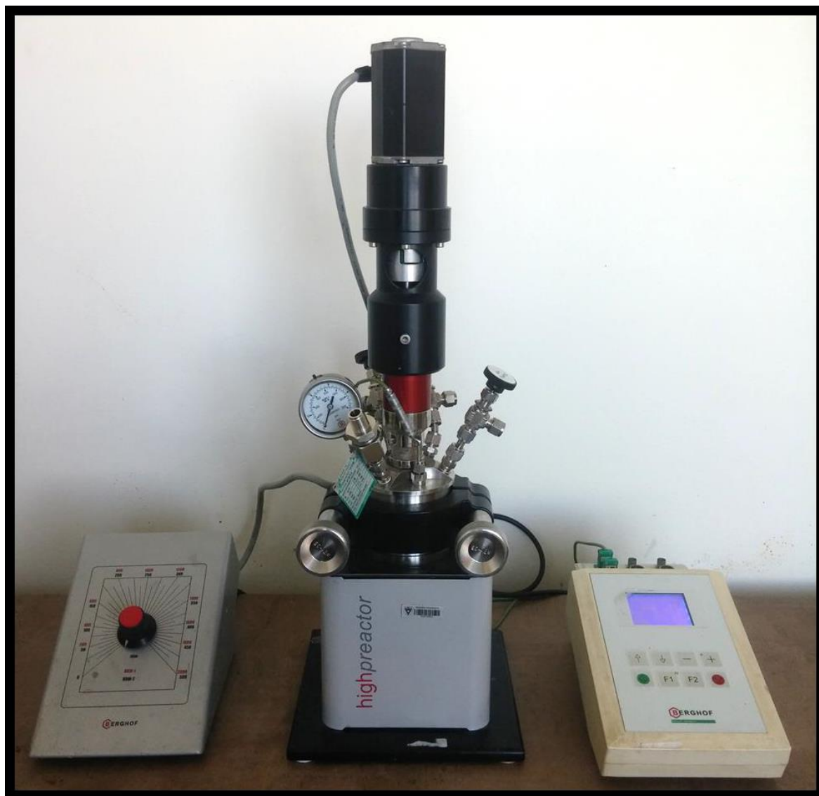
Figure 2.1. Berghof high pressure reactor employed for the hydrothermal synthesis of the QDs used in this work.
