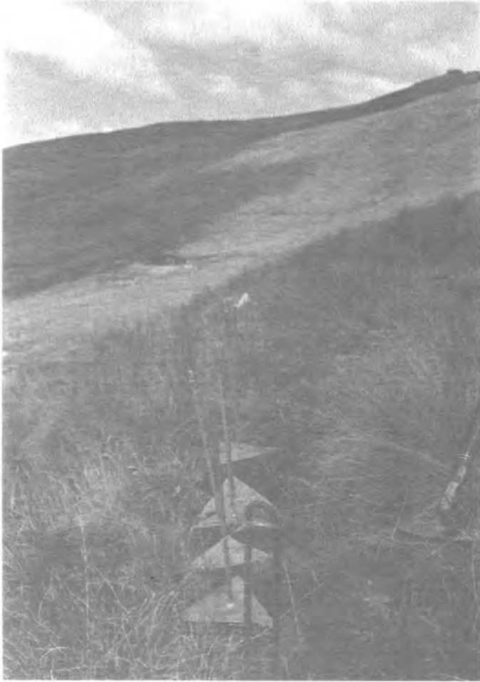
Figure 6.5: Downslope displacement of metal markers of lobe M2 in November 1996. The markers have moved out of line, and are also no longer flush with the ground surface due to frost heave.
