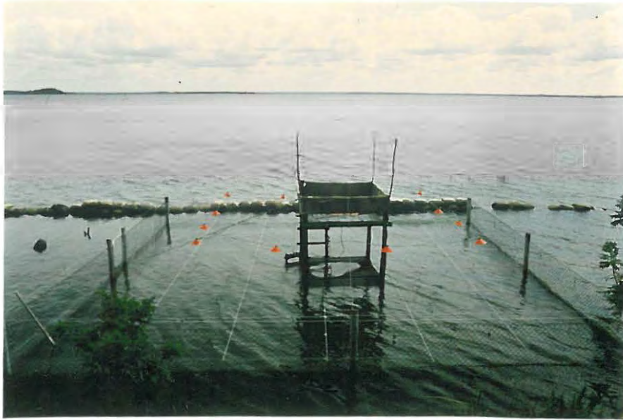
Figure 63A: Predation experimental area I (PEA I); showing central hide, red lights and above water cords dividing observation area into 36 equal squares.
