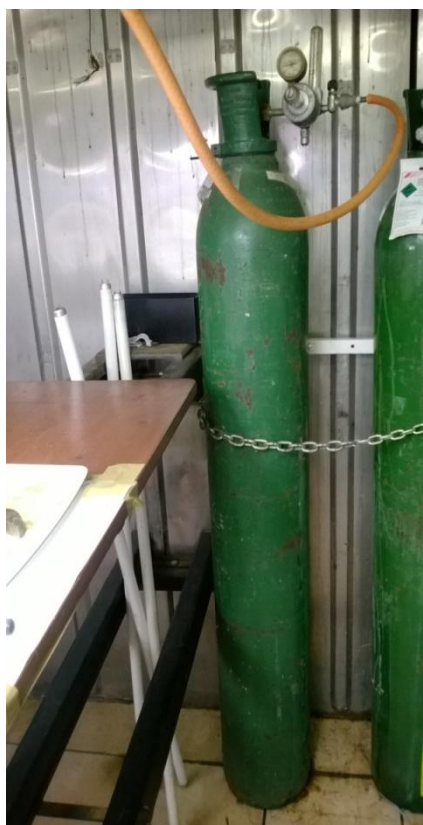
Figure 5.2 A compressed carbon dioxide (CO 2 ) gas cylinder with a CO 2 regulator.
