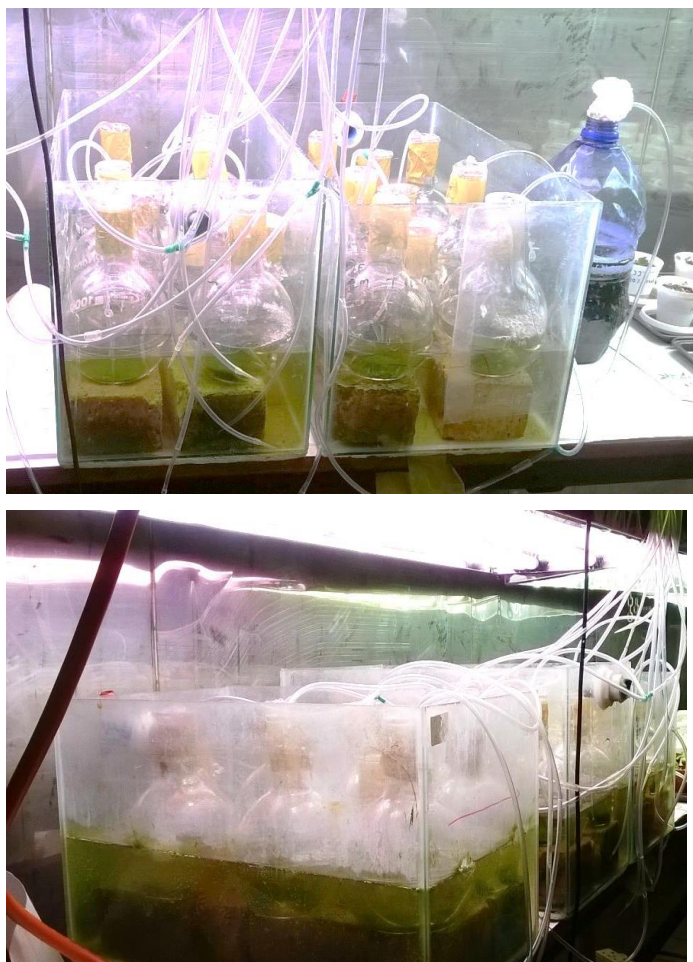
Figure 5.1 Glass tanks (water baths) with flasks containing microalgae culture.
