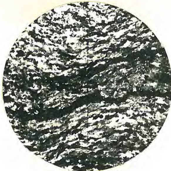
Plate XXIII : Slightly contorted flow-banding in the ankeritic beforsite. Magnetite and haematite (black), carbonate (grey and white). Polarized light, x 32.
