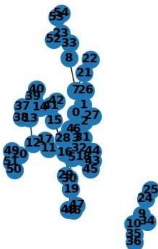
Figure 2.8: An example where the networkx library has separated the graph describing the molecule into two fragments, with each atom specified by number.
