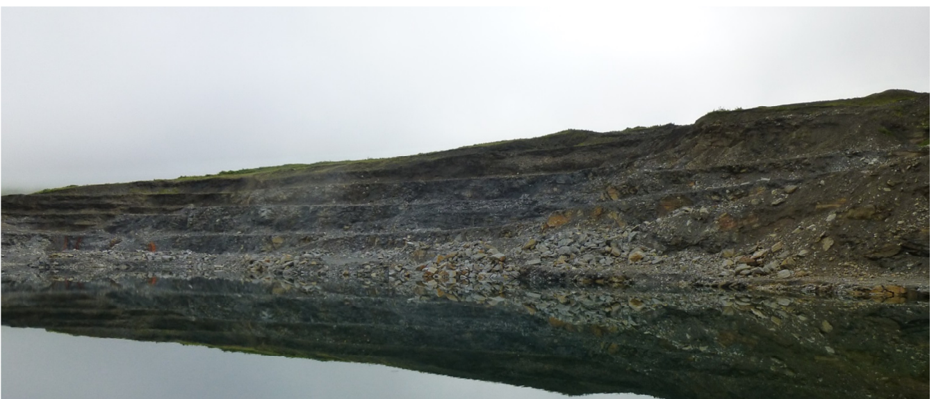
Figure 28: The Rock Creek Mine pit, now filled with water, has been developed in graphitic schists of the Devonian Dcs formation. Benches are ~3 m high.
