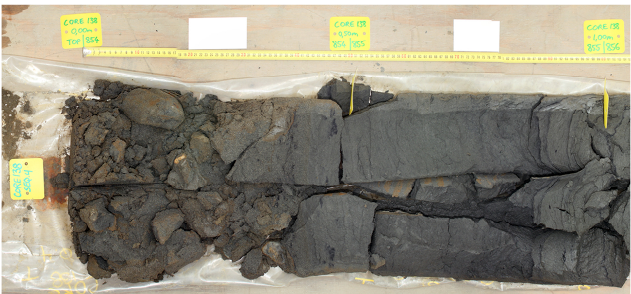
Figure 26: The top metre of Core 138. The top ~40 cm is dominated by a gravelly sand unit which overlies laminated glacial muds.
