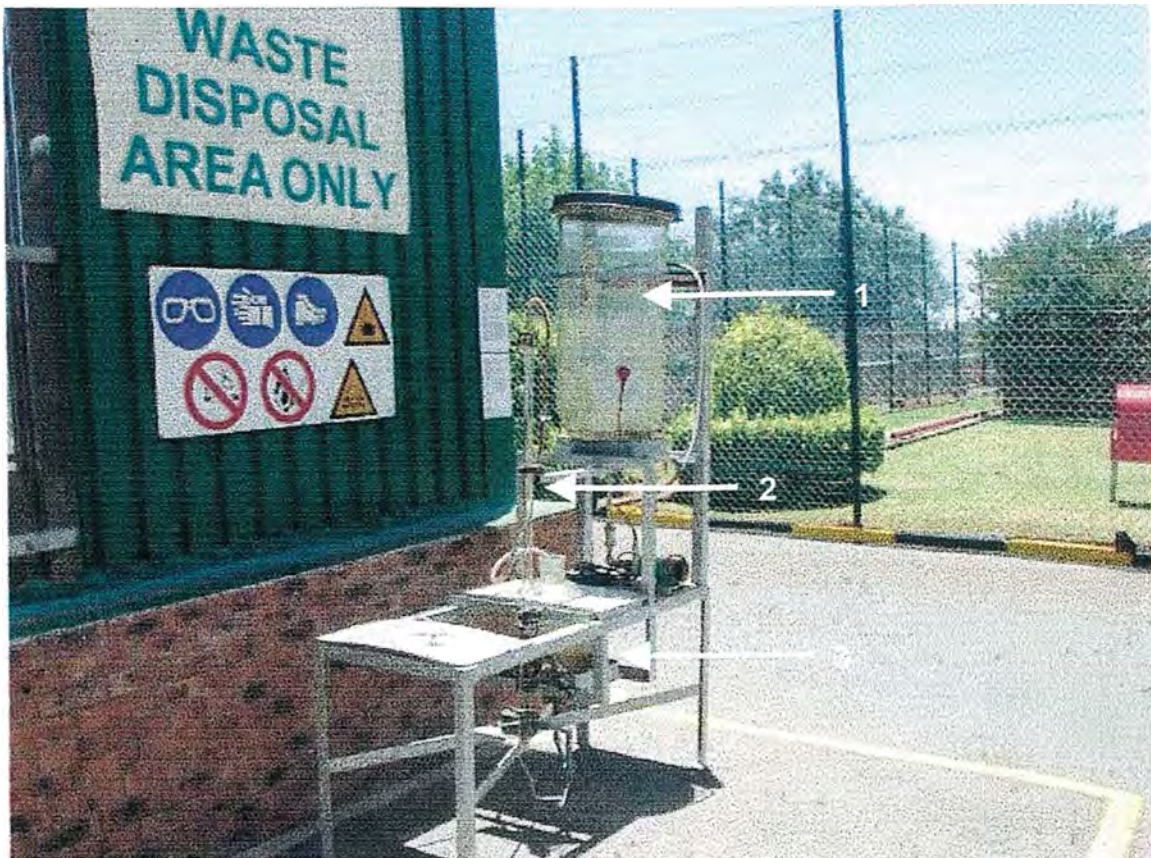
Figure 4.1: Up-flow construction of Rig 1.
