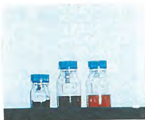
Fig 7.2. Hydrogen Sulphide Production and Media Discoloration due to Halotolerant and Halophilic Bacteria from Salted Hides after 28 Days Incubation
