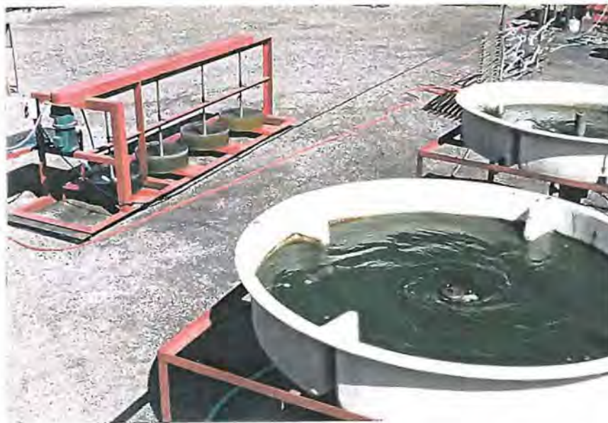
Figure 4.1 Culture units used for the determination of D. salina biomass productivities. Note the dark green colours of the algal cultures.
