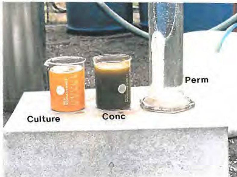
Figure 6.20 Air-displacement CFUF concentrate (4.3 g dry wt.l -1 ) and permeate. Starting culture density 0.4 g dry wt.l -1 .
