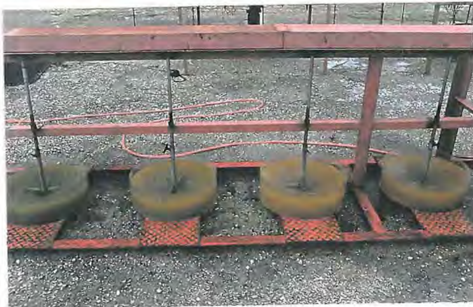
Figure 5.1 Multi-stirring unit used to mix the 0.2 m 2 stress ponds. Note the bright orange colour of the stressed cultures.
