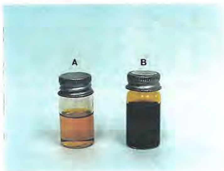
Figure 7.5 Difference in solubility of synthetic all- trans - \beta -carotene (A) and of the D. salina sterioisomeric mixture (B).
