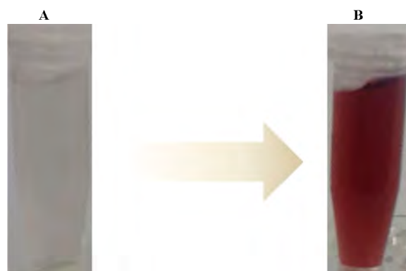
Figure 4.1: Synthesis of AuNPs by citrate reduction. (A) Aqueous tetrachloroauric acid (1.0 mM) and (B) reddish-brown colour indicating the formation of AuNPs after the addition of trisodium citrate (2 ml; 1%).
