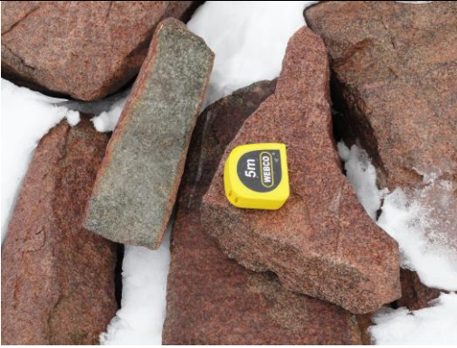
Figure 12: Oxidised surface and weathering rind observed on a sample rock for the blockfield. Note the red surface compared to the grey rock.
