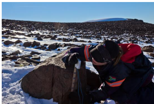
Figure 20: Clinometer affixed to wooden support when taking dip measurements in the field (Photo: van den Berg, 2012).
