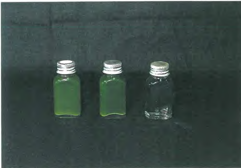
Figure 9.6 Cell concentrate (1.5% SDW) and permeate produced by CFUF concentration of D. salina .
