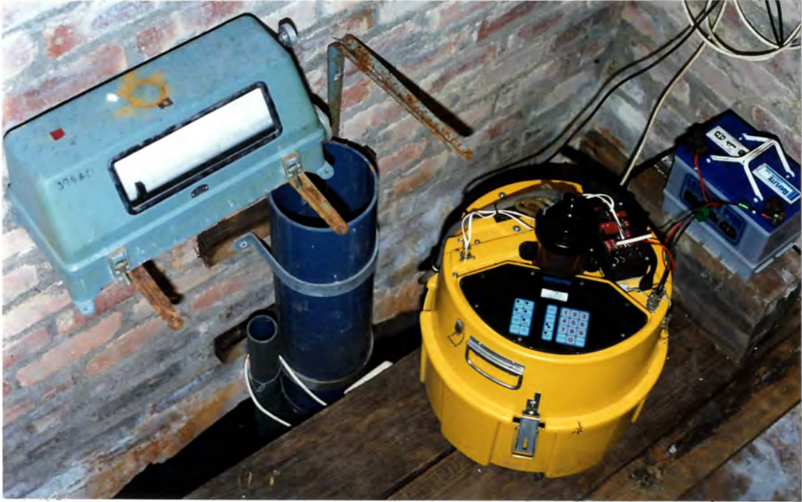
Plate 4 The Pond 6 "manhole" monitoring site showing the flow gauging system and automatic water quality sampler
