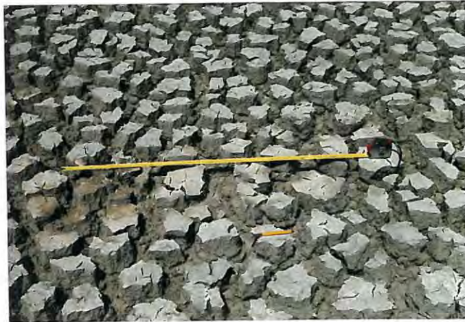
Plate 7 The filter mat which formed on the deepest portion of the basin floor. On drying 15 cm deep cracks/crevices formed
