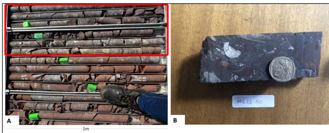
Figure 15: Drillcore images from farm McCarthy containing eastern belt Mn ore , shale-hosted breccia and the Blinkklip breccia. A. The red square marks the occurrence of the Blinkklip breccia as well as its transition into the red shale-hosted breccia in drill core MC35; B. A typical hand specimen of the Blinkklip breccia.
