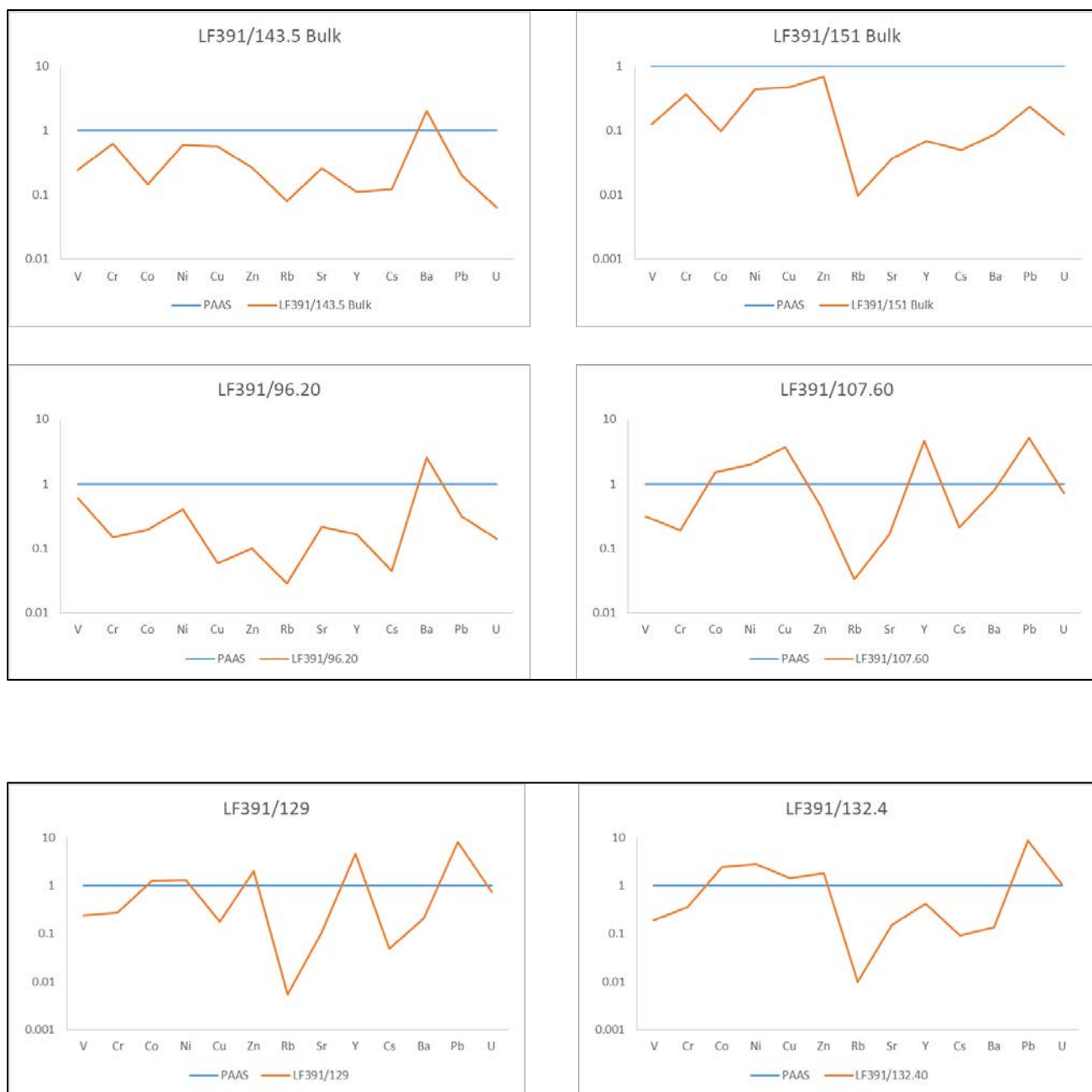
Figure C3: Ore trace elements from the Leeuwfontein locality plotted against PAAS
