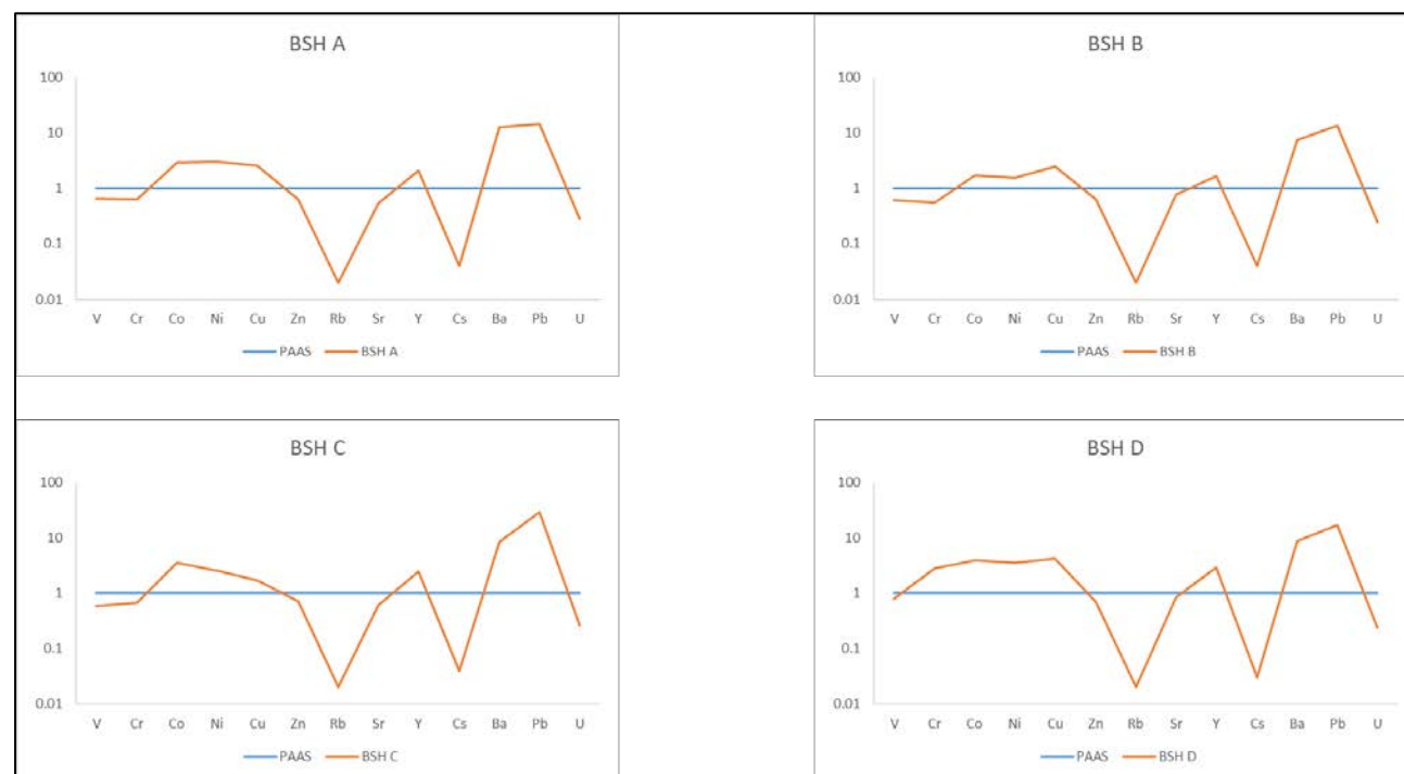
Figure C1: Ore trace element from the Bishop locality plotted against PAAS
