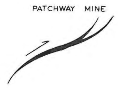
Overthrusting resulting in the development of secondary footwall spur veins.
