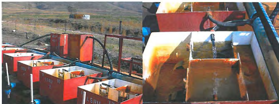
Figure 2.4: Splitter boxes at the VCC pilot plant showing the different feed compartments.
