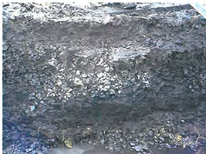
Figure 2.17: Depth profile of the waste material packed in SSRU 3 showing the evidence of heavy compaction.
