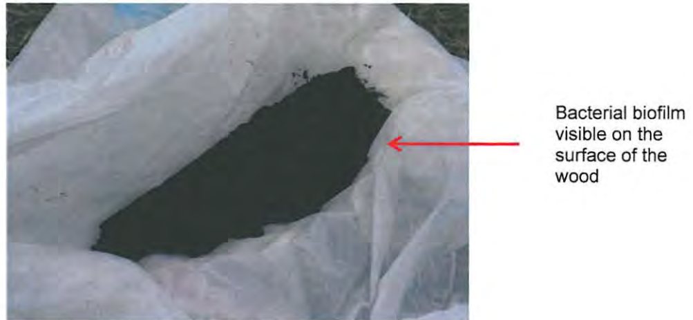
Figure 2.18: A block of wood recovered during decommissioning of the SSRU 3. It was noted that the wood serving as a carbon source in the reactor had not degraded after 6 years, however, there was distinct development of bacterial biofilm.
