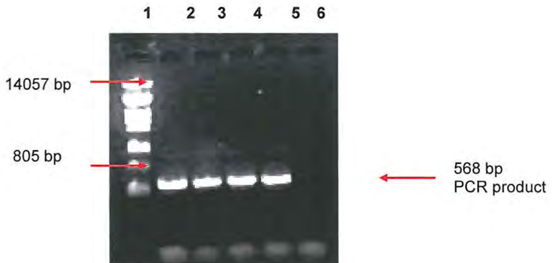
Figure 5.2 Agarose gel electrophoresis of 568 bp product. Lane 1: molecular marker \lambda pst ; lane 2–4: 568 bp PCR product amplified from total genomic DNA isolated from laboratory-scale column packed-bed reactor (lane2: inlet zone, lane 3: middle zone, lane 4: outlet zone); lane 5: positive control (568 bp construct); lane 6: negative control.
