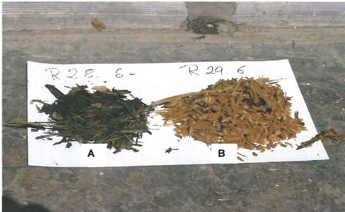
Figure 3.7: Organic matter from the middle sections of two reactors. (A): reactor under investigation, (B): poorly performing reactor.
