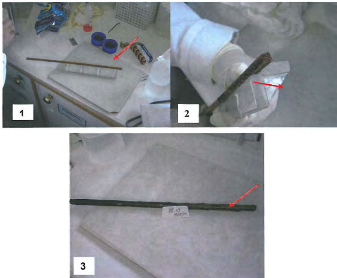
Figure 2.31: Discoloration and biofilm formation on wood sampling rods at different stages: (1) After one month, (2) after four months, (3) after six months. Red arrows point to the bacterial biofilm developed on the sampling rods.
