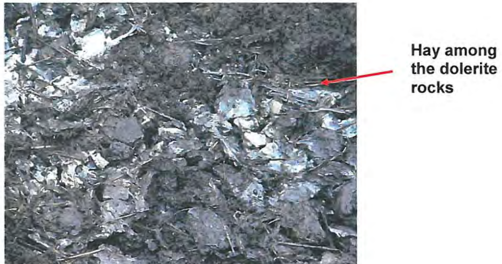
Figure 2.20: A layer of hay between the dolerite showing clearly that the material was not degraded over a period of six years of operation.
