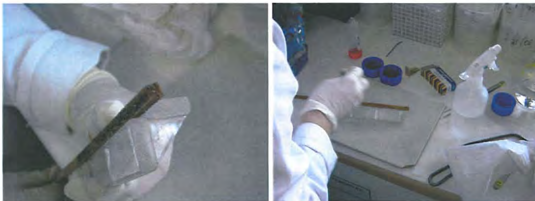
Figure 2.26: Sampling of biofilm growth which had developed on the wooden rods drawn from the column at regular sampling intervals.
