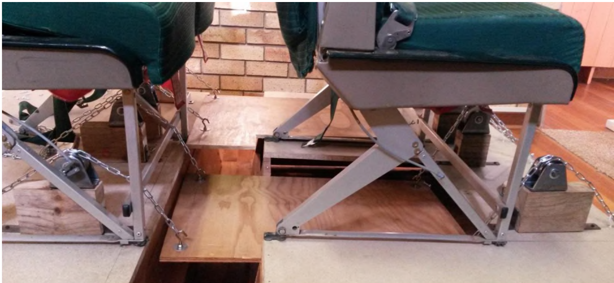
Figure 7: The pulley system devised to adjust the height of the aircraft chairs by altering the height of the floor.
