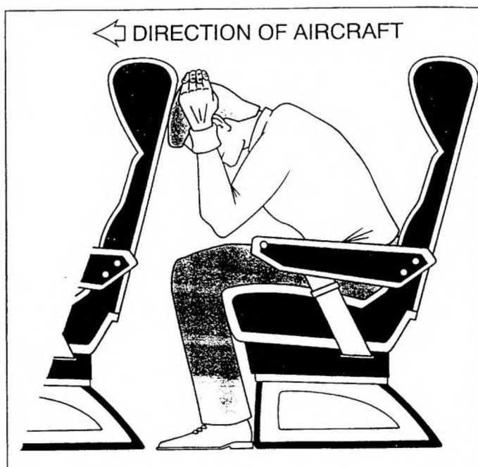
Figure 5: Recommended crash brace position (Quigley et al. , 2001).
