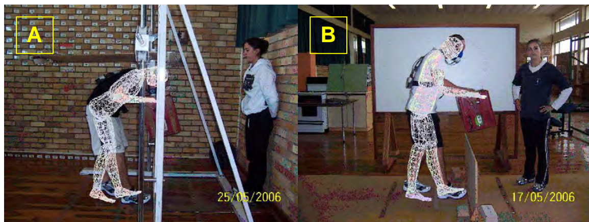
FIGURE 7: Lifting postures adopted during the lifting action in (A) the restricted and (B) the unrestricted tasks.
