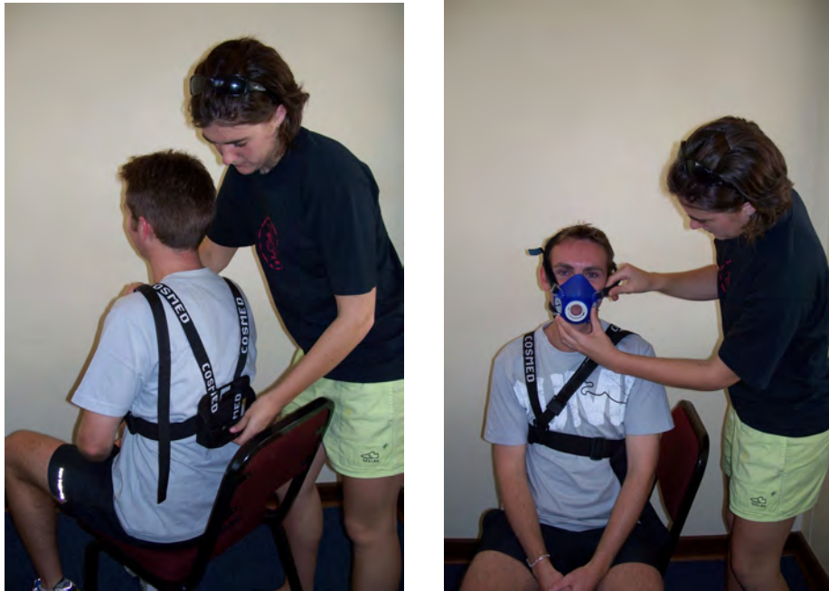
FIGURE 3: An assistant attaching the Cosmed K4b 2 ® to a recruited subject.
