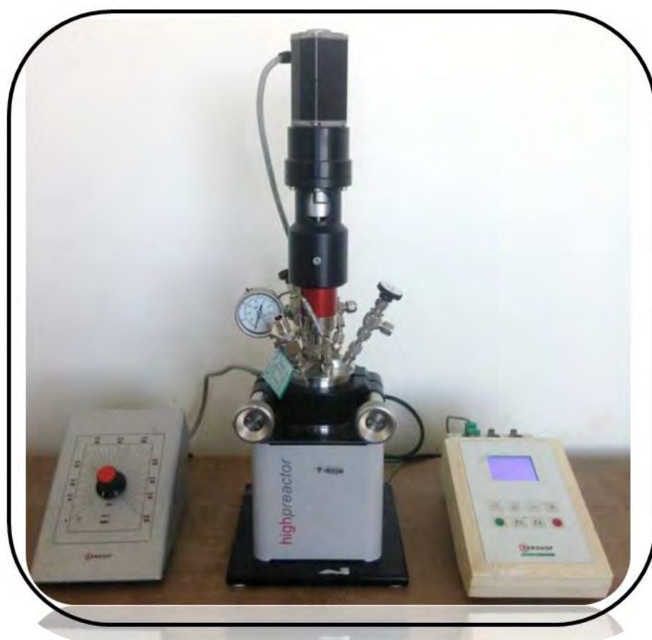
Figure 2.1: The Berghof high pressure reactor, autoclave used for the hydrothermal synthesis of GQDs and NGQDs
