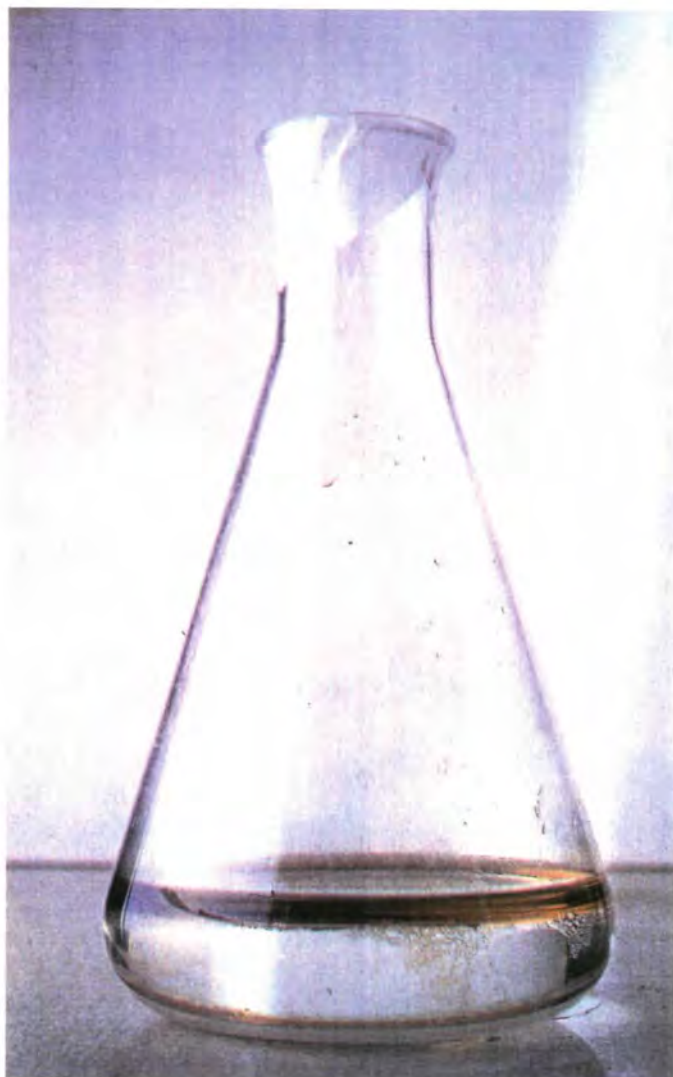
Plate 5.5: The formation of a brown precipitate above the solvent during enzyme catalysis in an aerated organic medium using crude tyrosinase.
