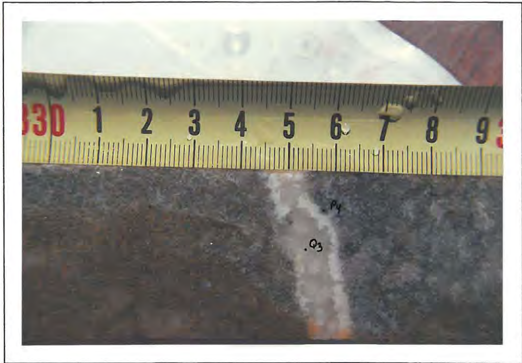
Figure 40. A typical example of the phyllic alteration (69,66 - 69,74m) within the RDP2 core. The quartz and pyrite alteration are clearly seen. Qz = quartz and Py = pyrite.
