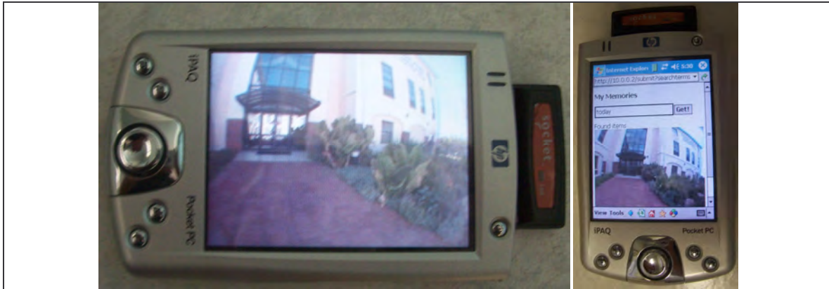
Figure 54. PDA based memory retrieval interface showing live video from the wearable camera using [CoreCodec, 2005] and the onboard PDA web browser being used to retrieve memories from the memory manager through the HTTP based memory browser
