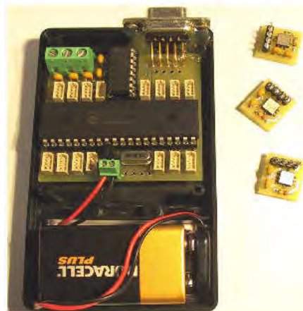
Figure B8. Laerhoven's PWM multiple sensor analogue to digital convertor package [Laerhoven, 2002]
