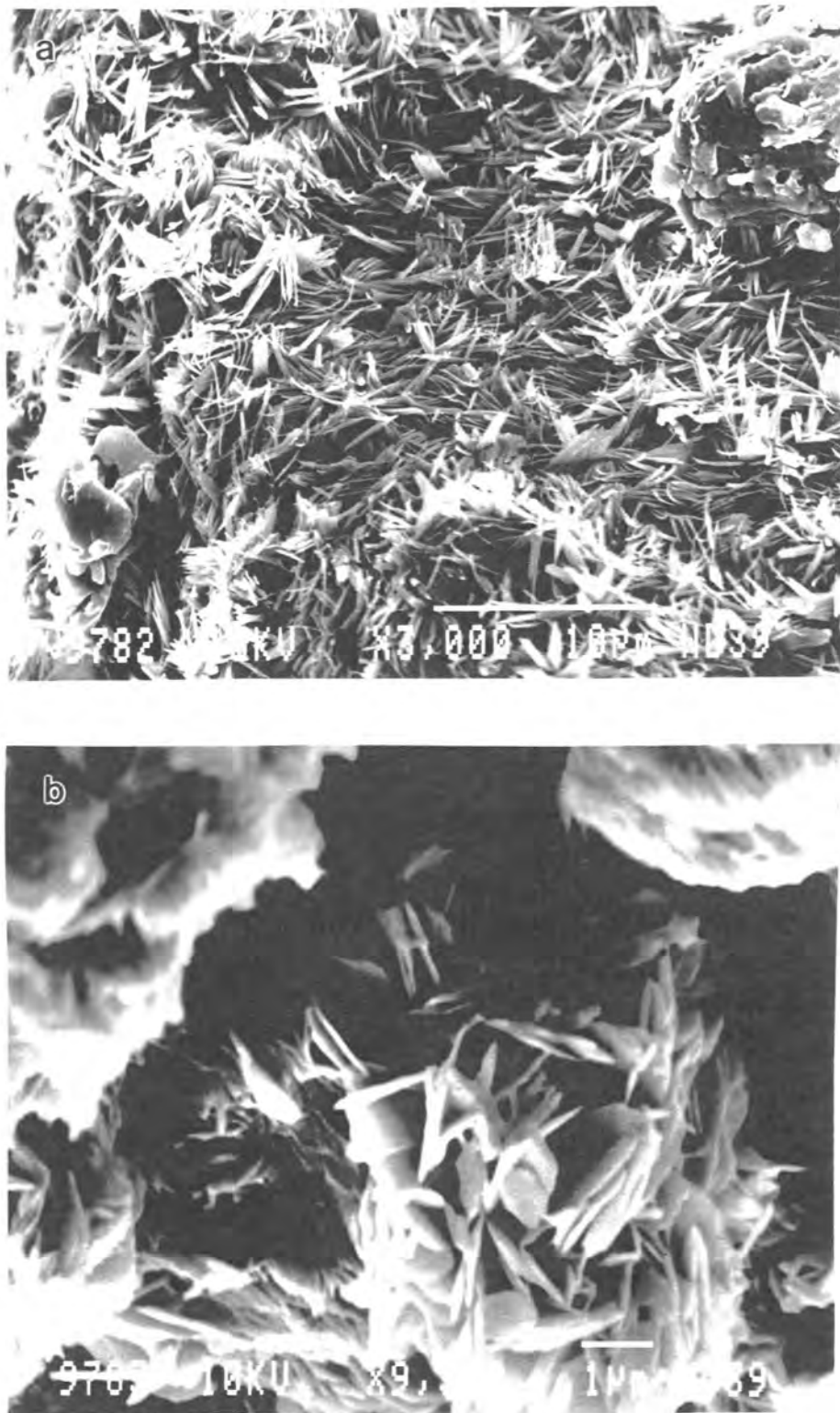
Figure 9.3: High magnification scanning electron micrographs of the surface of grains of granular biosorbent, x 3 000 (a) and 9 500 (b) magnification. Note the crystalline flakes which supply a very large surface area.
