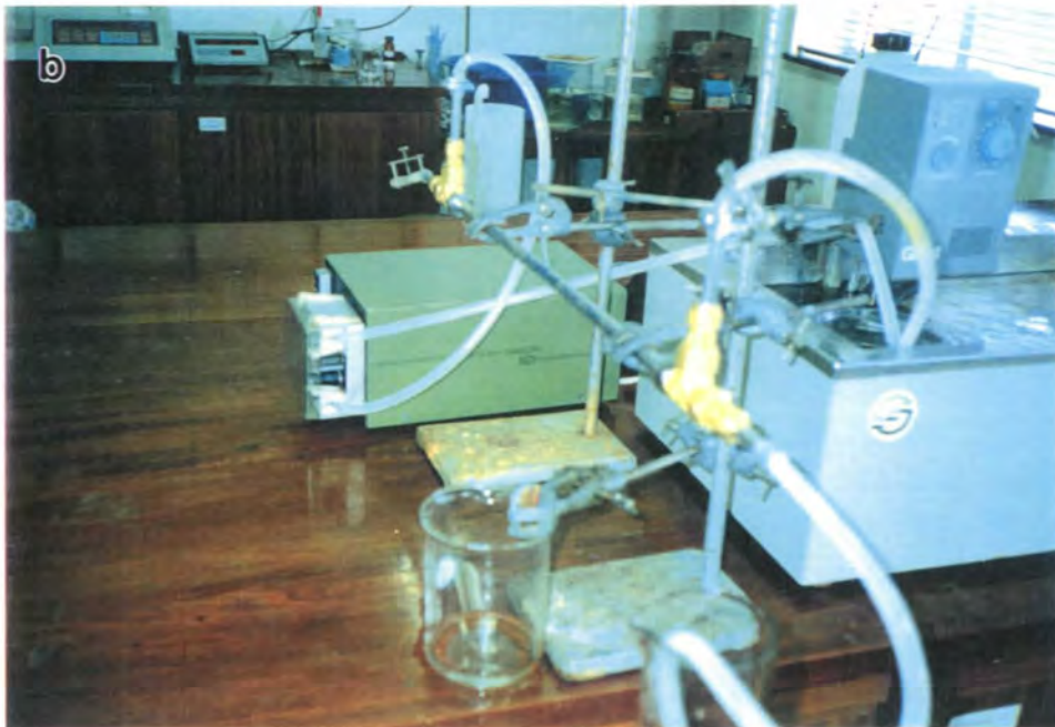
Figure 3.4: Microfiltration equipment set-up, both schematically (a) and a photograph of the actual cross-flow microfiltration system used (b). There were 7 hollow fibres within the cartridge with a total surface area of 0.013 \text{ m}^2 .
