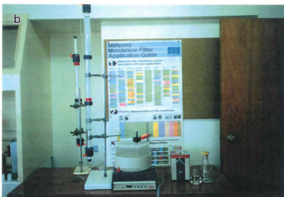
Figure 15.1: Varian Techtron 1000 atomic absorption spectrophotometer (a) and KLB chromatography columns (b) which were used during the present study.
