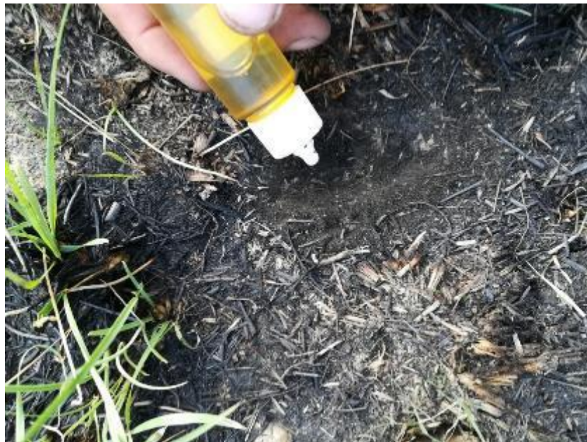
Figure 3.4: Water Drop Penetration Time test being carried out in the field at a recently burned sampling site.
