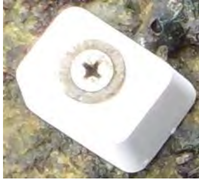
Figure 2. 5: Clod card fastened to the rock, used to quantify water motion over a 24-hour period.
