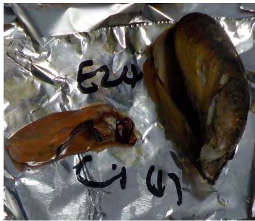
Figure 2. 4: Shell (on the right) and soft tissue (on the left) of a dissected mussel, placed on pre-weighed aluminium foil which was then dried in the oven.
