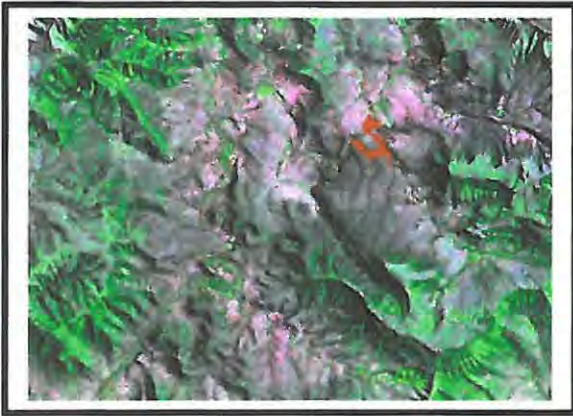
Figure 5.1: Assignment of red to band 3, green to band 4 and blue to band 5.
