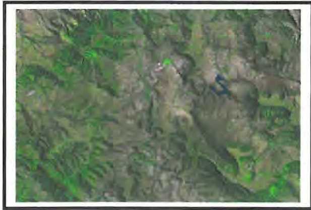
Figure 5.2: Assignment of blue to band 3, green to band 4 and red to band 5.
