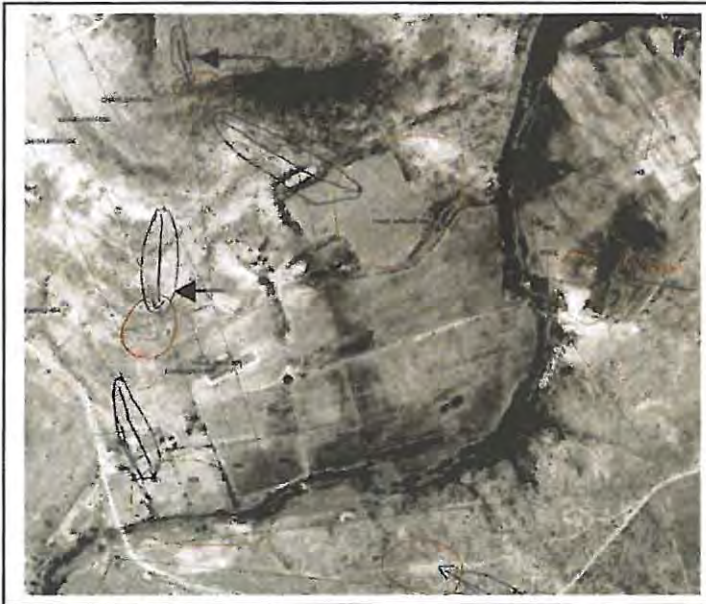
Figure 8.7: These delineated gulleys and areas of contributing flow (indicated by arrows), are placed down the line of a ridge. The remaining gulleys represent the areas defined at the mapping workshop.
