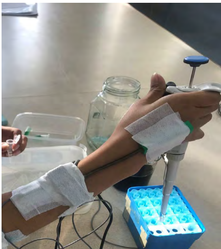
Figure 12: Placement of Bi-axial goniometer on pipetting hand.
