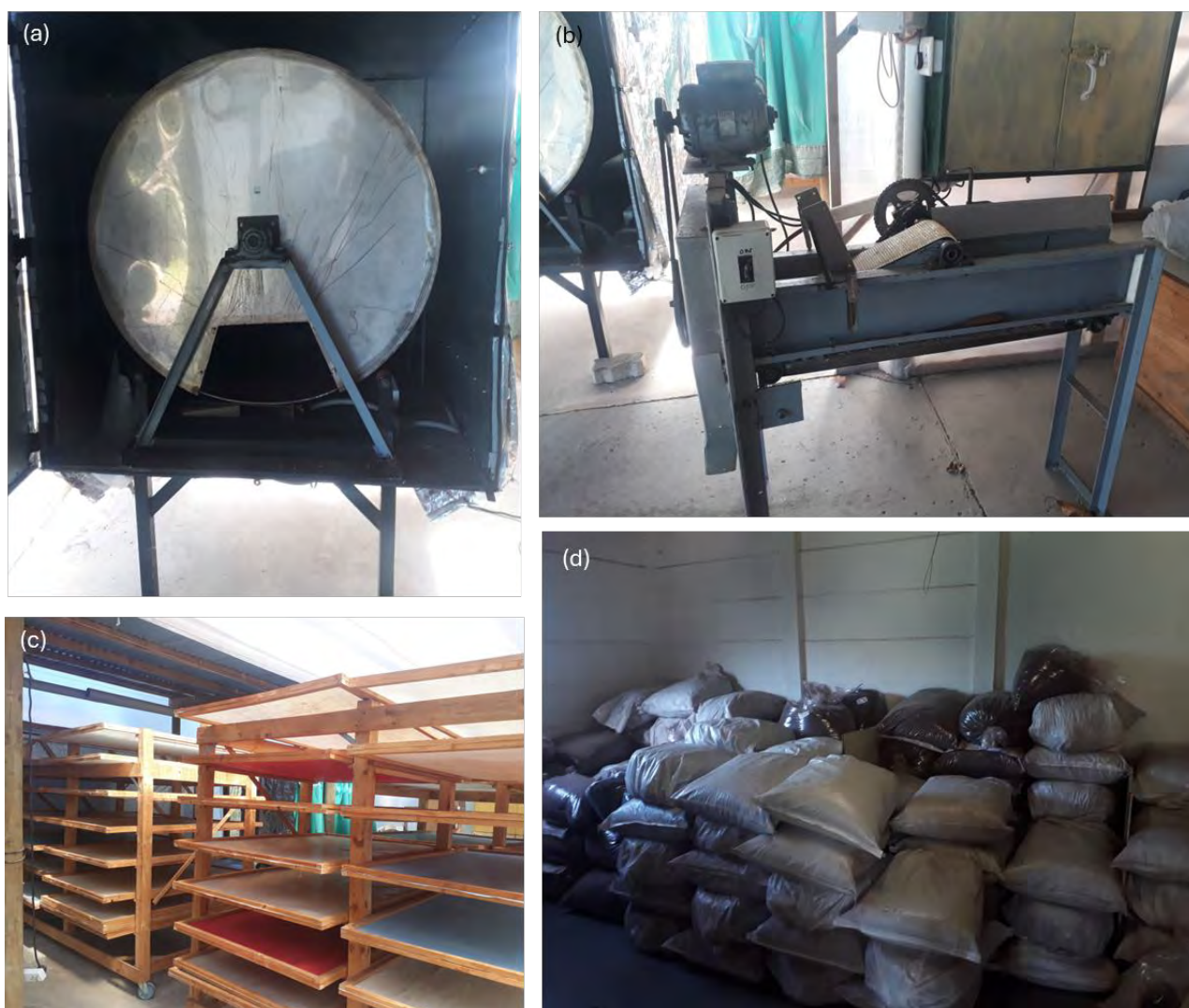
Figure 24: Honeybush tea processing facility at Enterprise 3, which was built by the owner. It includes a (a) furnace; (b) tea cutter; (c) tea drying racks; and (d) a storage facility housing all the processed products in bags in the storage facility.
