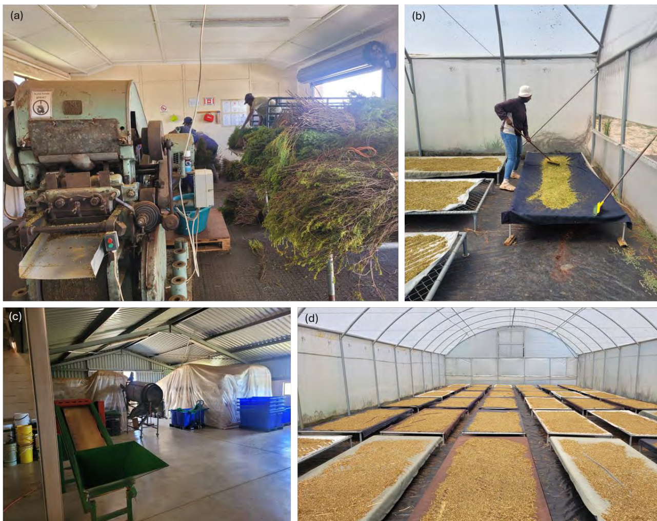
Figure 23: Honeybush tea processing facility at Enterprise 1. (a) Staff are feeding bundles of wet honeybush tea material into the tea cutter to be cut into different sizes; (b) Student (Tafadzwa Makhuza) is seen spreading freshly cut honeybush tea on the drying racks; (c) Well-maintained equipment and processing compliant; (d) Honeybush tea that is drying on drying racks.
