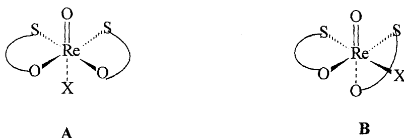
Figure 4.11. Two possible molecular configurations of Re(V)-oxo complexes with bidentate acylthiourea ligands.
