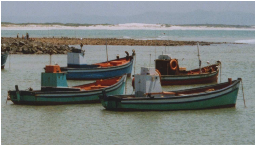
Figure 2. Chukkies, the smaller (8 - 10 m) wooden vessels moored in a small boat harbour in the southwestern Cape.
