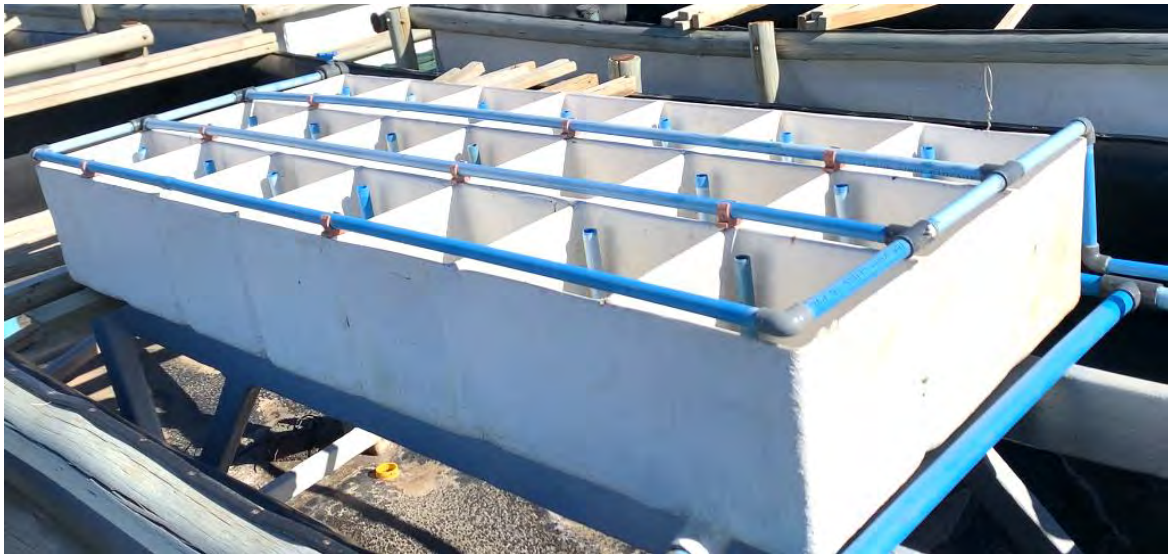
Figure 4.1: The tank setup for temperature and sediment experiment. Only two of the three rows of tanks were used (n=14 tanks).
