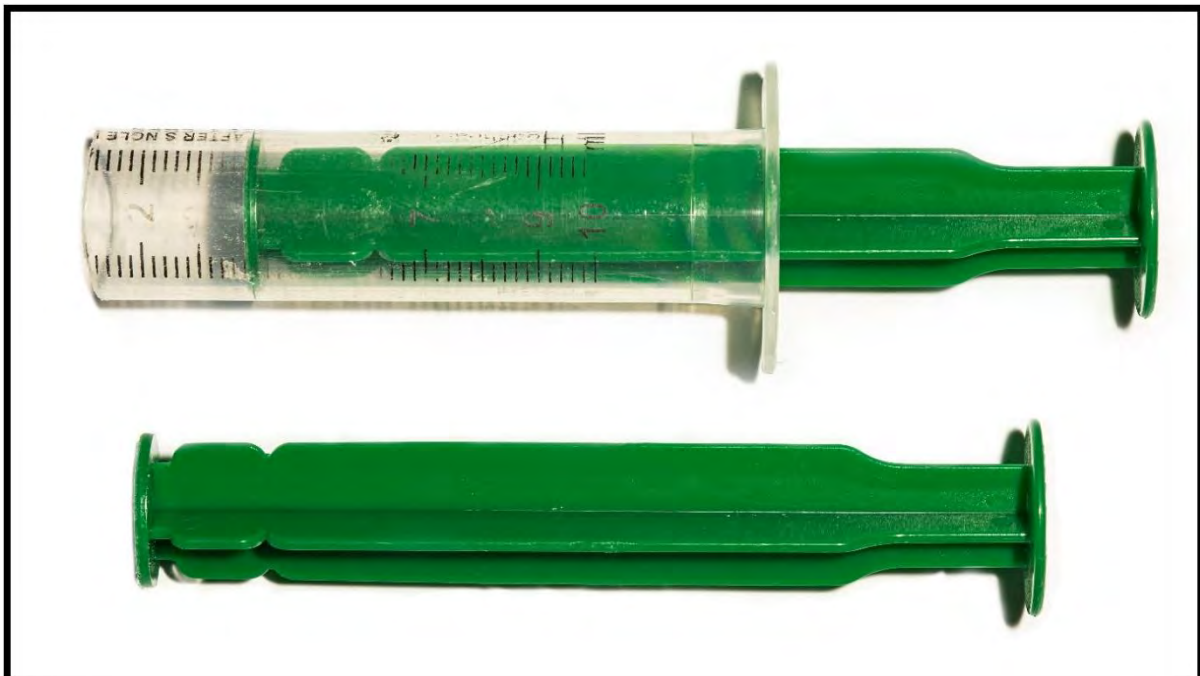
Figure 4.1. Modified 10 mL syringe used for cutting diet (top) and syringe piston used for compressing diet into wells and vials.
