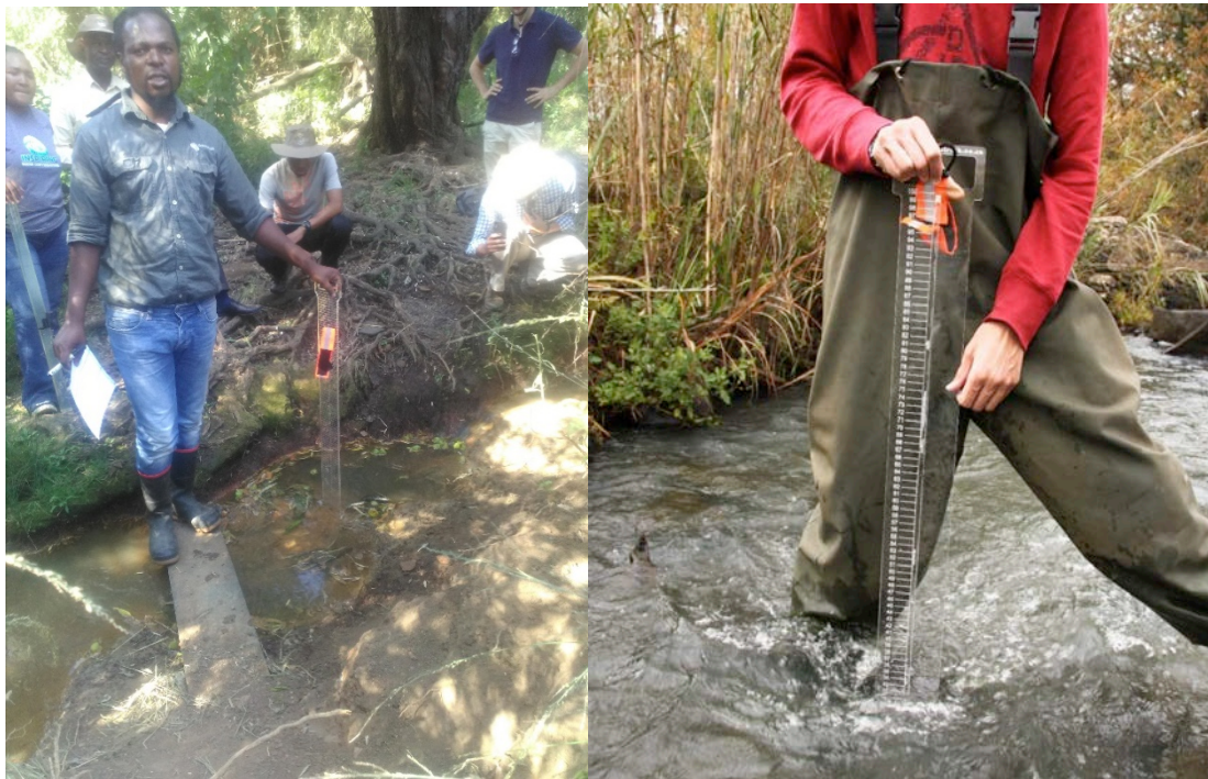
Figure 7.5: Transparent velocity head-rod. Left: Held by Ayanda Lepheana during the demonstrations. Right: A closer look at the transparent velocity head-rod (WRC, WESSA, and GroundTruth)
