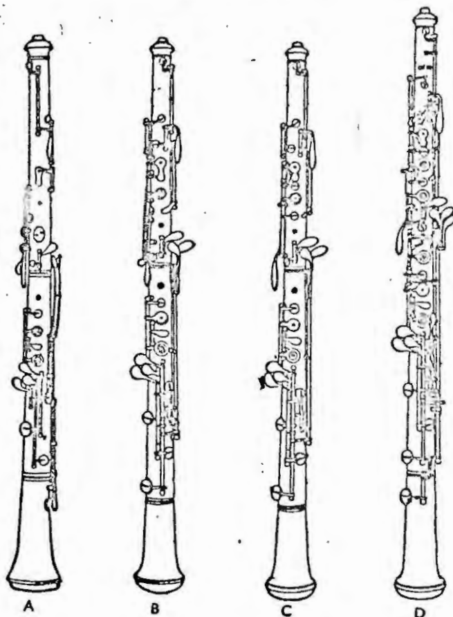
A. Typical French Oboe, c.1840. B, C and D. Triébert's Systèmes Nos. 4, 5 and 6.
