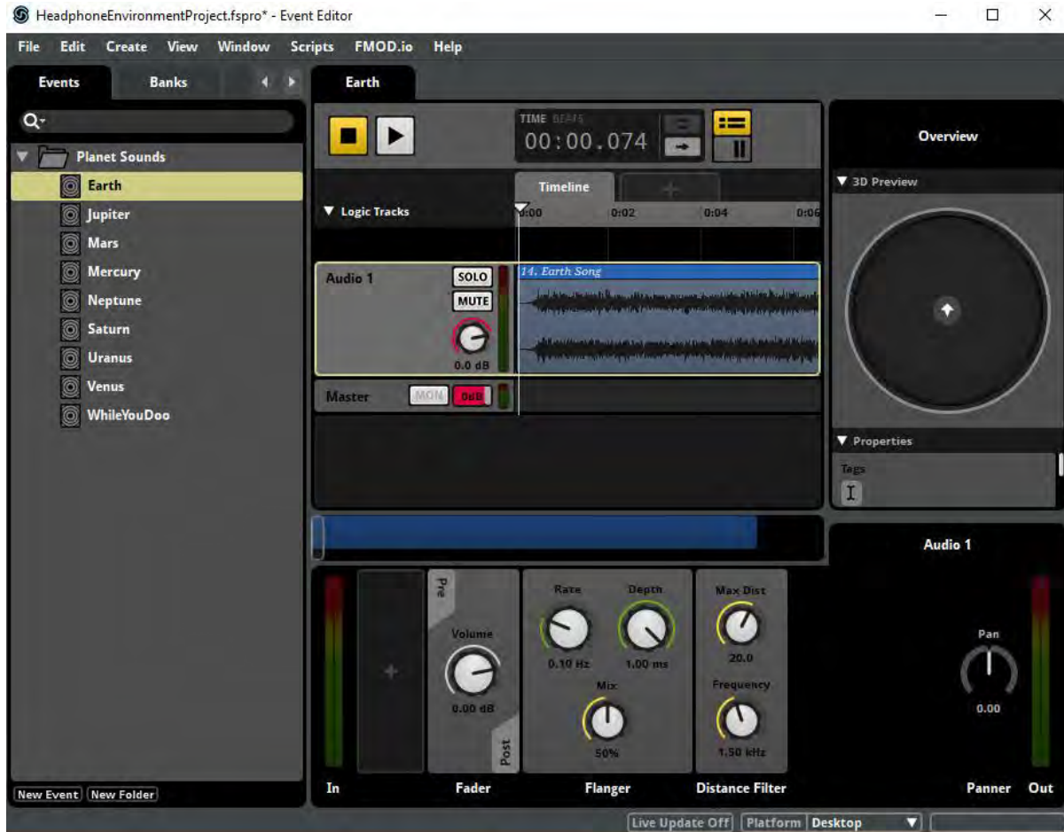
Figure 143: This screenshot shows an overview of a FMOD audio event within the FMOD Studio Application. The specific event (“Earth”) has a few DSP effects on its DSP chain (Fader, Flanger, Distance Filter).
