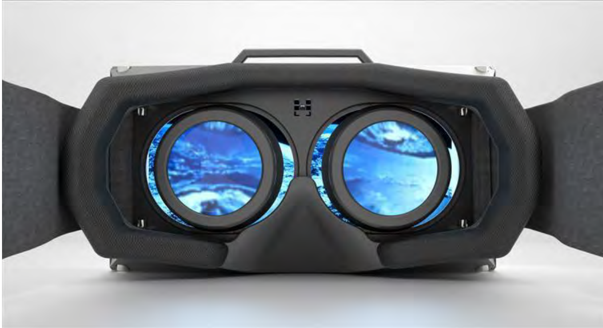
Figure 12: An image that shows the internal display and screens used for the Oculus Rift Development Kit 2 (Goradia, et al., 2014).
