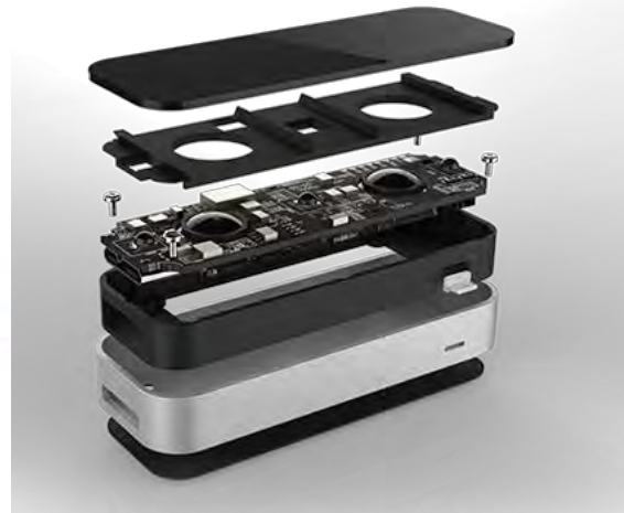
Figure 13: The left picture of the leap motion controller indicates the right-handed coordinate system it employs. 12 The right picture shows the different layers of the device. 13
