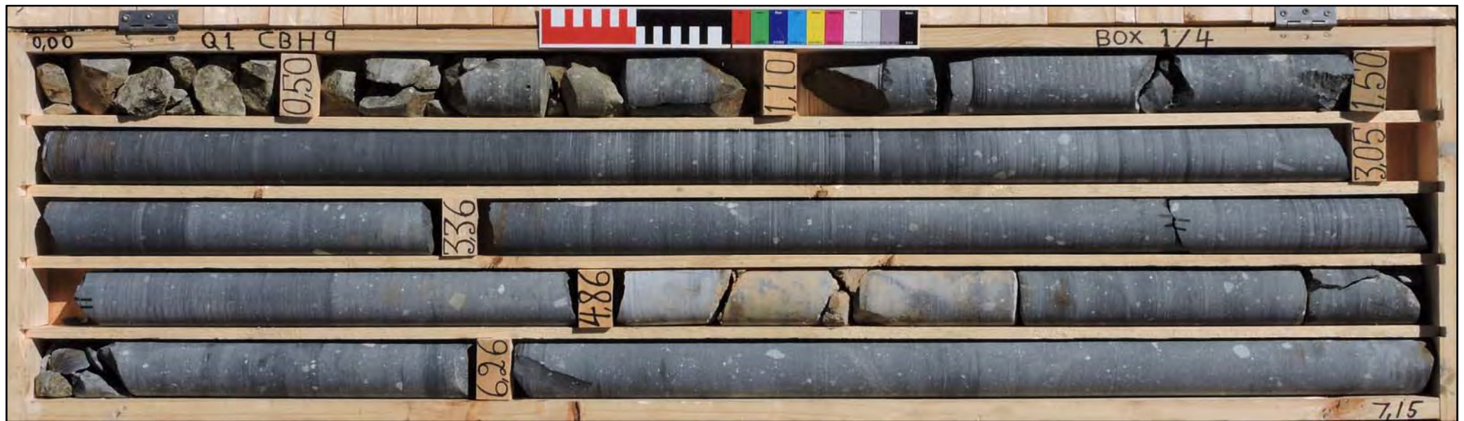
Figure 4.4: Typical tillite drill core recovered from geotechnical borehole
