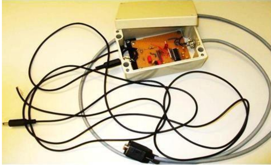
Figure 3.7: Constructed CI-V level converter, illustrating the CI-V jack that connects to the transceiver and the DB9 connector that connects to the computer's COM port
