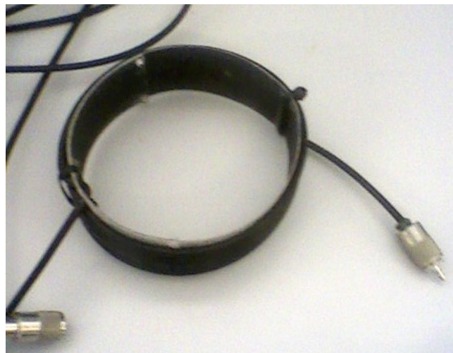
Figure 3.3: Constructed HF choke balun, showing the coaxial cable wound on the PVC ring.
