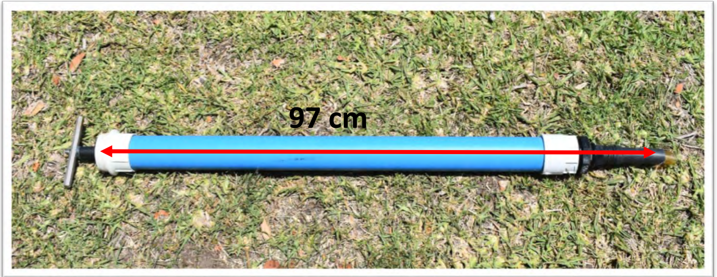
538 Figure 2.6. Modified manual suction pump system adapted from the design of Gulliksen & Derås 539 (1975) used to collect all epibenthic macrofauna found within the crevices and on top of the Reno 540 mattress structures.
