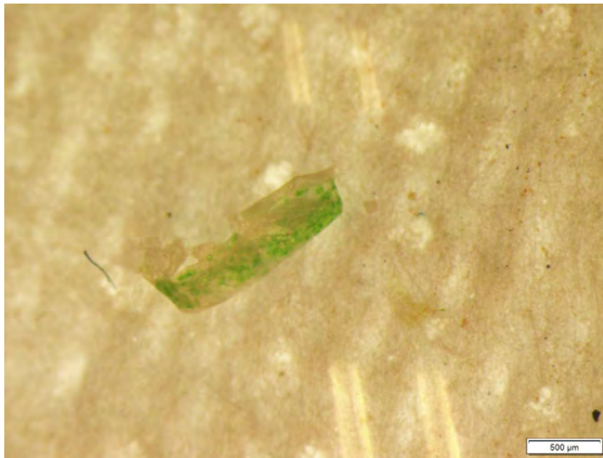
Plate C11. Polypropylene film (FTIR spectrum indicated as alphabet 'e' in Appendix B2, Figure B2)
