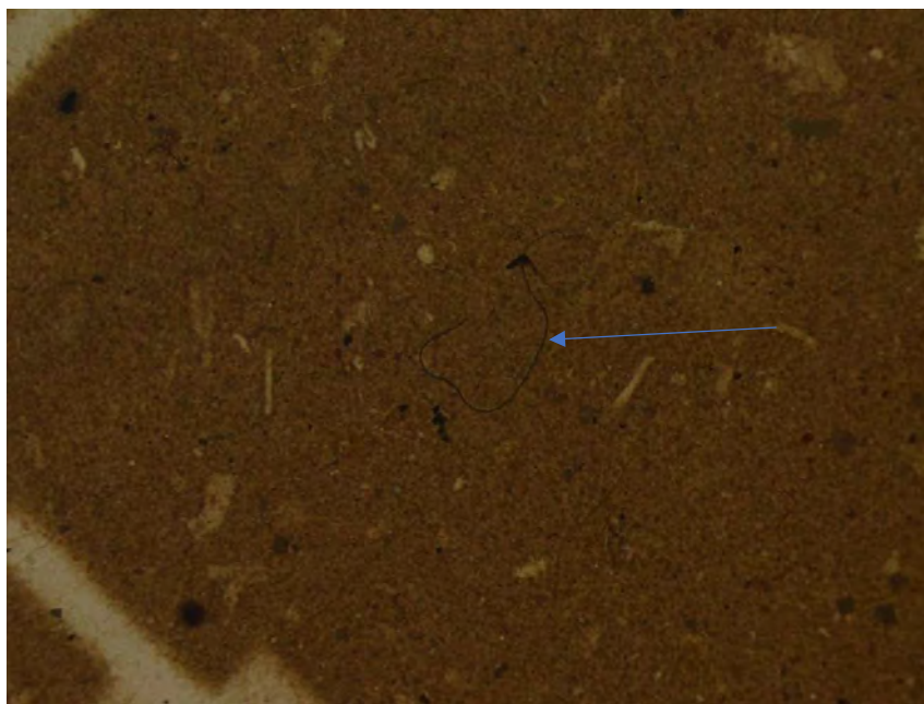
Plate C5. Polyethylene fibre (FTIR spectrum indicated as alphabet 'e' in Appendix B, Figure B1)
