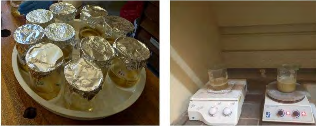
Figure 2.14. Samples prepared for digestion (left) and digestion on magnetic stirrer (right)
