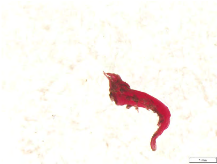
Plate C3. Polyethylene fragment (FTIR spectrum indicated as alphabet 'c' in Appendix B, Figure B1)
