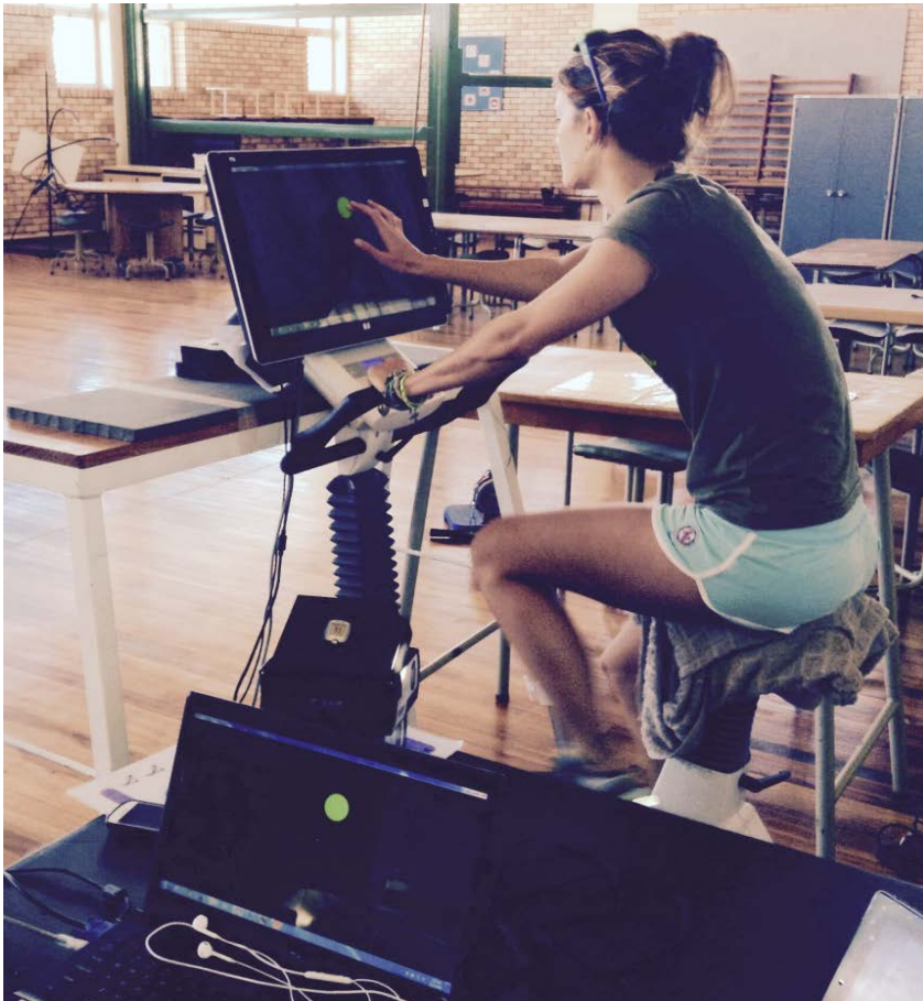
Figure 7. An image showing a participant performing the modified Fitts' task while cycling on an ergometer
