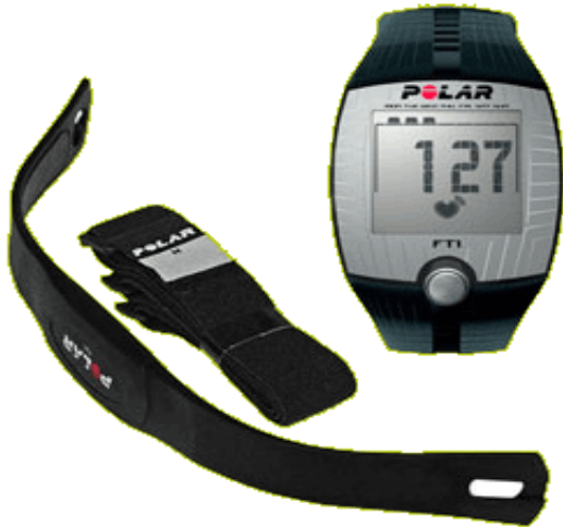
Figure 8. An illustration of the heart rate monitor that was used in this study. (Left: heart rate belt or chest strap with a wireless transmitter; Right: wrist watch receiver with a digital display)
