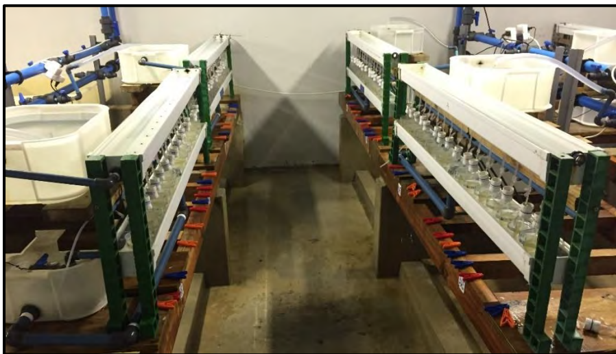
Figure 2.7: Four of the five experimental systems designed and built for the trials carried out for this thesis. This figure depicts the system prior to larval inoculation, when plates were being treated – as indicated by the multicoloured pegs which were used to mark plates and their respective treatments after randomisation had been carried out.
