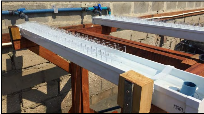
Figure 2.5: Experimental settlement plates at the start of a conditioning period. Shade cloth covers were removed during winter, as diatom overgrowth was less likely to occur during periods of shorter daylength.
