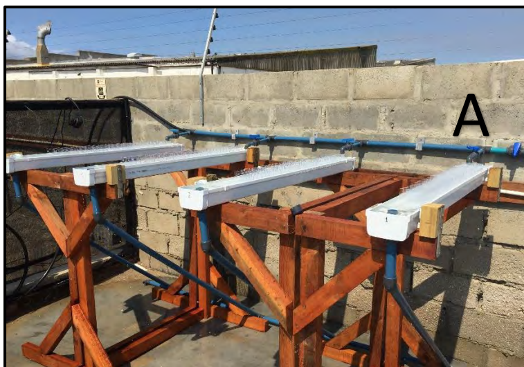
Figure 2.4: The ambient biofilm conditioning troughs were placed in a well-lit area of the farm to facilitate diatom growth. The shade cloth covers had not yet been attached to the frames at the time this photograph was taken. (A) indicates the mounted pipe line to supply water for the troughs and rinsing hose.
